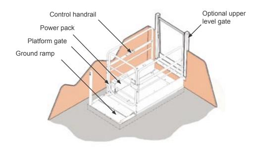
The lift is suitable for internal and external locations and a major feature of the design is that the platform is free standing, eliminating the need for guide column supports and thus minimising aesthetic intrusion into the environment. The majority of the lift is finished in brushed stainless steel finish. Other finishes can be supplied to special order.
