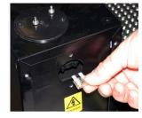
b) In the event that the lift malfunctions part-way through its travel it can be lowered by swivelling to one side (after removing one posi-drive screw) the round plastic cover on top of the box on the platform and pressing the black button. Remember to replace the cover and screw afterwards.
