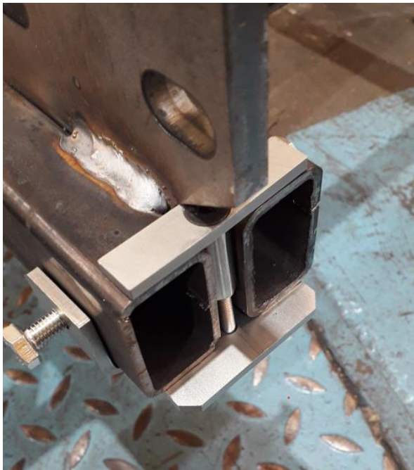
Clamp extension bracket assembled to platform to increase engagement between pit prop and underside of platform.
