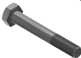
M10 x 70 hex head bolt, grade 8.8, BZP - ISO 4014 (4 off)
