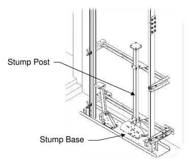
During installation, it is sometimes necessary to install packers below the stump post. These packers should be located on the **lower** plate of the stump base, with the stump post sitting on top of the packers.
