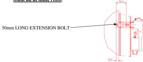
BOLT ENGAGEMENT INTO DOOR MUST BE AT LEAST 7mm
