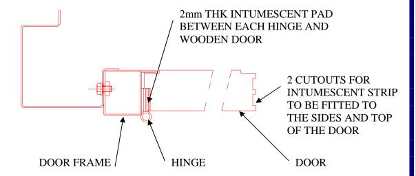
Intumescent strips should be fitted to the two routed channels on the sides and top of the door. **Both sets of strips** are required to be fitted to ensure the fire seal is not compromised.
