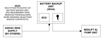
An RCD will be installed by Stannah within the battery backup enclosure. It is connected such that during a fault to earth the RCD will isolate the lift from both the mains incoming supply **and** the battery backup supply.
