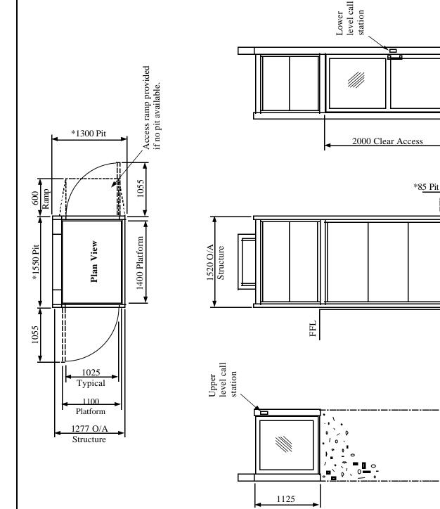
Vertical Lifting Platform Specification Complies with BS 6440 300Kg Single speed electro-hydraulic 0.1m/sec nominal
