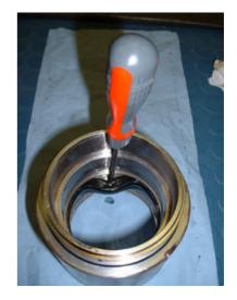
When the old seal has been removed, clean the housing thoroughly and check for any damage to the machined surface or debris left inside.
