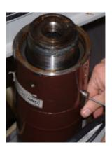
Clean the exposed ram thoroughly and check for anything that could damage the new seal whilst it is being replaced.
