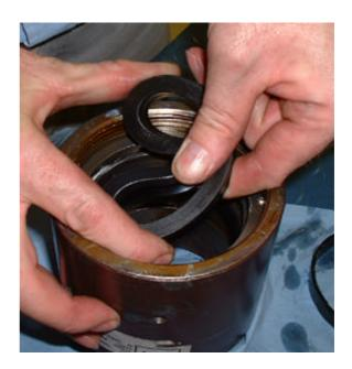
Before the seal housing is re-fitted, lubricate the seal and ram with some hydraulic oil, replace the "O" ring seal between the seal housing and cylinder and reassemble in the reverse order to removal.
