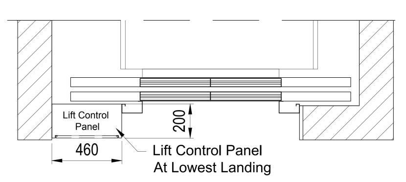
Lift Control Panel must be located at bottom floor only, next to the landing entrance
