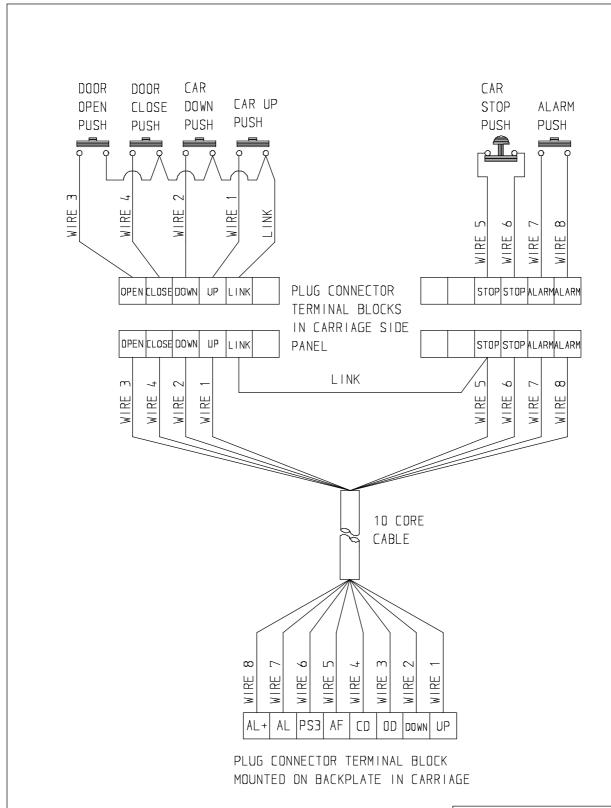
DRAWN: D. CLARK DATE: 19/1/98 WIRING FOR PANEL MOUNTED PUSH BUTTONS IN CARRIAGE USING LOOMS
